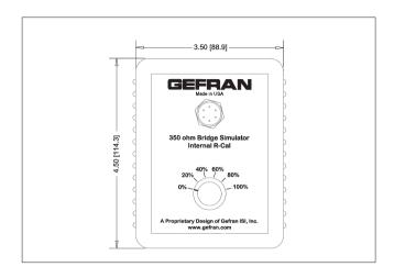
The TS3 simulates the output of a Gefran mV/V melt pressure transducer (M3 and W3 series) at various pressure levels.
